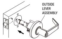
Install outside lever assembly on the door. Make sure tail of latch engaging with retractor correctly as illustration left.
